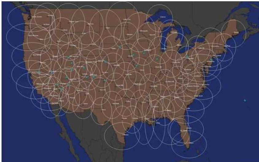
Figure 21. Aircell provides the backhaul for WiFi service on planes via a network of EVDO base stations (depicted as circles) on the ground. From http://www.aircell.com/index.php?option=com_content&task=view&id=312&Itemid=1
